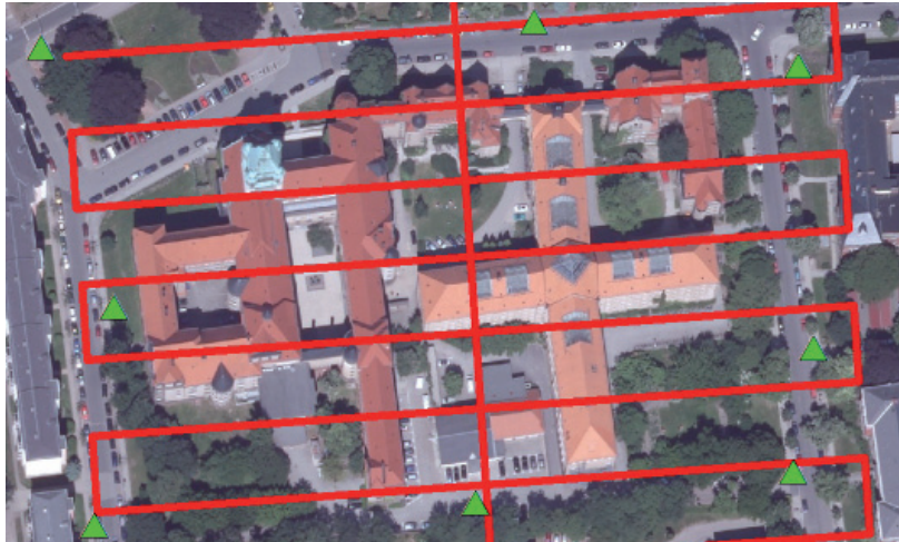
Planned flight path (red) and positions of control points (green triangles) data source orthophoto: ATKIS®-DOP © Staatsbetrieb Geobasisinformation und Vermessung Sachsen 2013 (GeoSN)
