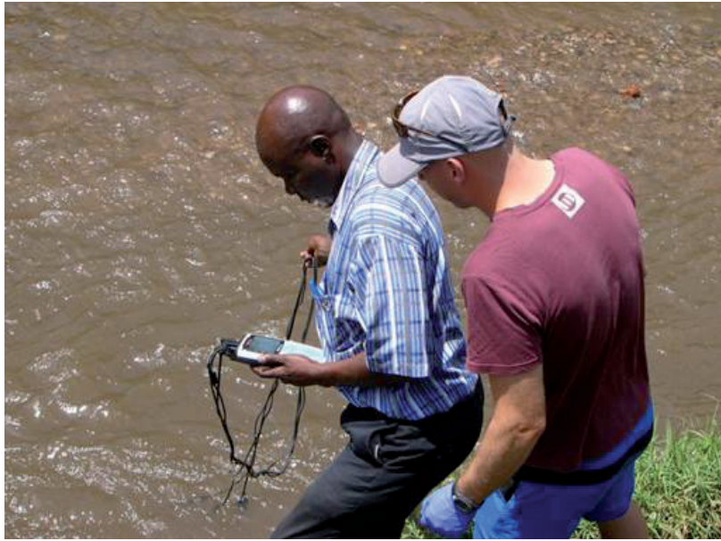
Taking in situ measurements of the physical properties such as water temperature
