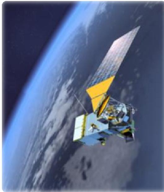
**AVHRR** (Advanced Very High Resolution Radiometer) is a broad-band scanner, sensing in the visible (red), near-infrared, mid infrared and thermal infrared portions of the electromagnetic spectrum, carried on **NOAA**'s (National Oceanic Atmospheric Administration) Polar Orbiting Environmental Satellites (**POES**) and more recently also on the European **MetOp** satellite.
